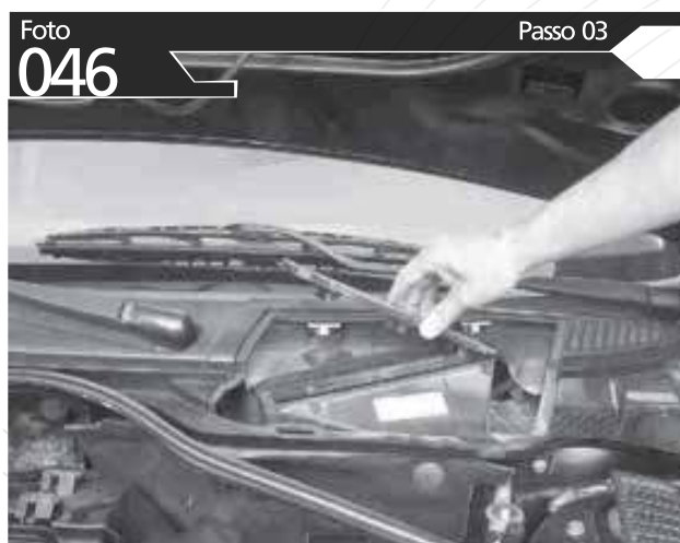
DESPARAFUSE E RETIRE A TAMPA
